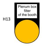
Indicator light – supply plenum box filter of the paint booth is clogged
